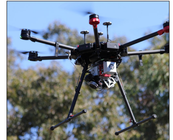
DJI Matrice M600 equipped with RIEGL miniVUX-SYS using RIEGL Integration Kit 600
