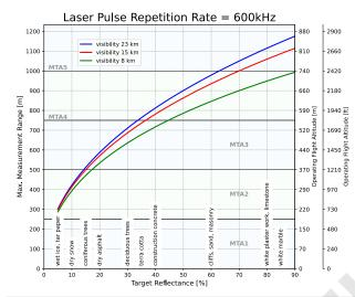
Operating Flight Altitude AGL given for the following conditions: FOV 75°, ambiguity resolved by multiple-time-around (MTA) processing, average ambient brightness, target size  $\geq$  laser footprint, roll angle  $<\pm 5$  deg
