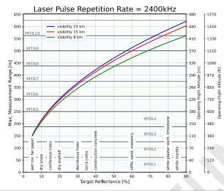
Operating Flight Altitude AGL given for the following conditions: FOV 75°, ambiguity resolved by multiple-time-around (MTA) processing, average ambient brightness, target size  $\geq$  laser footprint, roll angle <±5 deg
