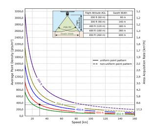
Example: VUX-180<sup>24</sup> at 1,800,000 pulses/sec, laser power level 100% altitude 600 ft AGL, speed 30 kn, resulting point density ~ 346.3 pts/m<sup>2</sup>
