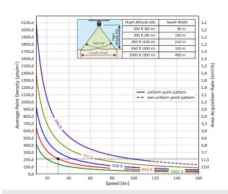
Example: VUX-180<sup>24</sup> at 1,200,000 pulses/sec, laser power level 100% altitude 650 ft AGL, speed 30 kn, resulting point density  $\sim 213.1~\text{pts/m}^2$
