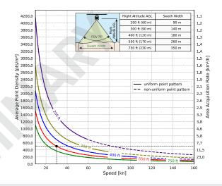
Example: VUX-180<sup>24</sup> at 2,400,000 pulses/sec, laser power level 100% altitude 550 ft AGL, speed 30 kn, resulting point density ~ 503.7 pts/m<sup>2</sup>
