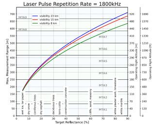
Operating Flight Altitude AGL given for the following conditions: FOV 75°, ambiguity resolved by multiple-time-around (MTA) processing, average ambient brightness, target size  $\geq$  laser footprint, roll angle <±5 deg
