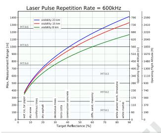
Operating Flight Altitude AGL given for the following conditions: FOV 100°, ambiguity resolved by multiple-time-around (MTA) processing, average ambient brightness, target size  $\geq$  laser footprint, roll angle  $\pm 5$
