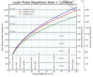
Operating Flight Altitude AGL given for the following conditions: FOV 100°, ambiguity resolved by multiple-time-around (MTA) processing, average ambient brightness, target size ≥ laser footbrint, roll angle ±5
