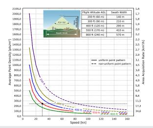
Example: VUX-16023 at 1,800,000 pulses/sec, laser power level 100% Altitude = 550 ft AGL, Speed 30 kn, resulting point density  $\sim 243~pts/m^2$
