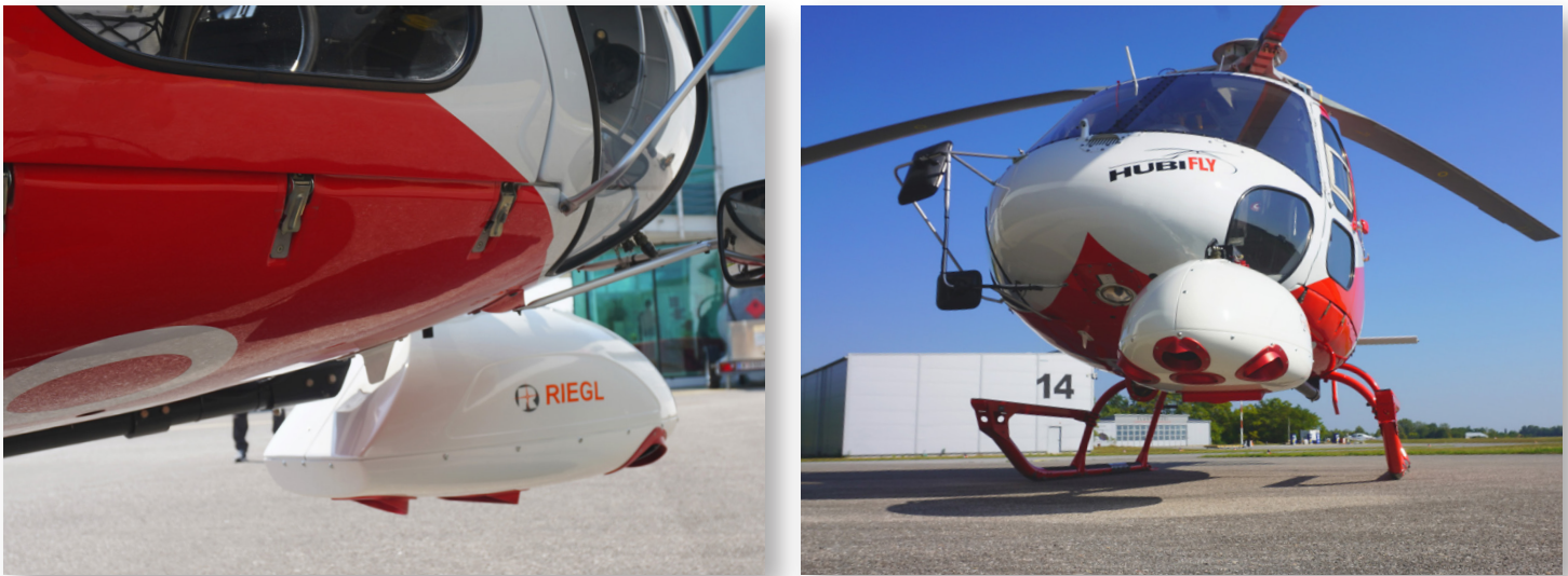
RIEGL's VQX-2 Helicopter Pod mounted to an Airbus Helicopters AS350.
