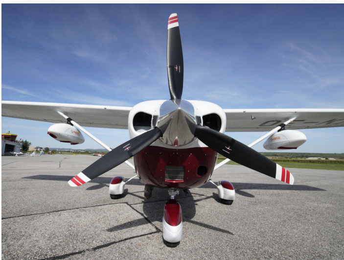
RIEGL's Cessna T206H test plane equipped with two VQX-1 wing pods
