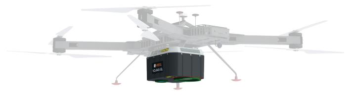
UAV integration example: RIEGL VQ-840-GL on a UAV-based platform
