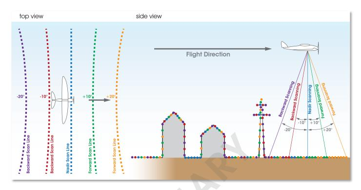
The *RIEGL* VQ-680 offers a sophisticated, multi-axis scan geometry consisting of five parallel scan lines per scanner rotation, but with each scan line having its own unique scan direction. The scan directions change consecutively from nadir, to +10 and +20 degrees forward, and to -10 and -20 degrees backward. This scan geometry provides superior coverage of vertical features ahead of and behind the sensor, creating best-of-class 3D LiDAR data sets.
