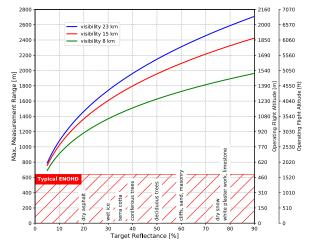
Example: VQ-680 at 1,800,000 pulses/sec, laser power level 100% Altitude =4,300 ft AGL, Speed 120 kn
