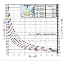
**Example:** VQ-580 II at 300,000 pulses/sec, laser power level 100% Altitude = 3,000 ft AGL, Speed 60 kn
