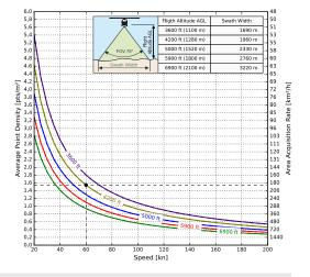
**Example:** VQ-580 II at 150,000 pulses/sec, laser power level 100% Altitude = 4,200 ft AGL, Speed 60 kn
