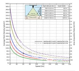
**Example:** VQ-580 II at 2,000,000 pulses/sec, laser power level 100% Altitude = 1,300 ft AGL, Speed 60 kn
