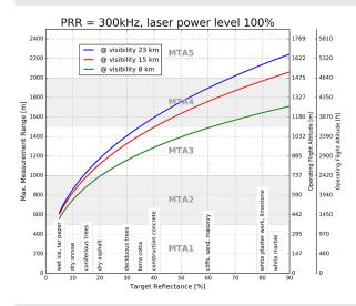
Example: VQ-480 II at 300,000 pulses/sec, laser power level 100% Altitude = 2,100 ft AGL, Speed 60 kn
