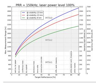
Example: VQ-480 II at 150,000 pulses/sec, laser power level 100% Altitude = 2,800 ft AGL, Speed 60 kn
