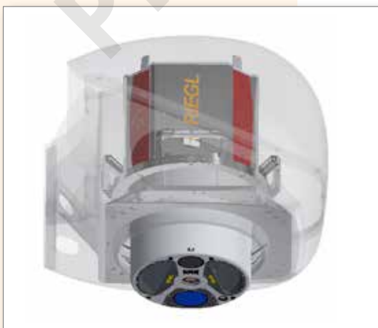
RIEGL VQ-1560 II-S installed in the nose pod of fixed-wing aircraft DA42 MPP
