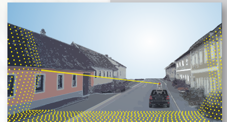
360° vertical field of view in a single pass
