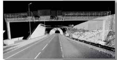
RIEGL VUX®-1HA scan data, transportation infrastructure mapping at highway speed
