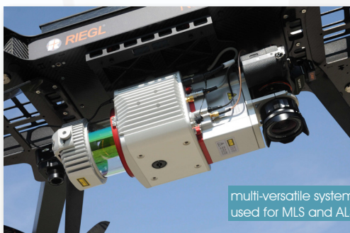
RIEGL VUX-1UAV LiDAR Sensor equipped with APX-20 UAV, Flir Tau 2 thermal camera, and Sony A7R III camera
