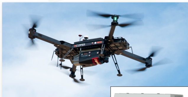
RiCOPTER with RIEGL VUX-240 LiDAR Sensor, APX-20 UAV and nadir RGB camera fully integrated
