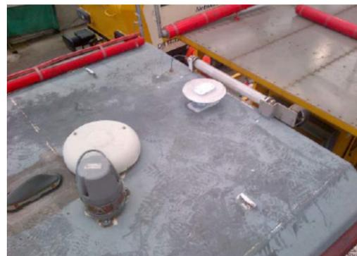
GPS Antenna installed on MPV
