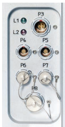
The Z+F PROFLER® 9012 with detailed view of the ports.
