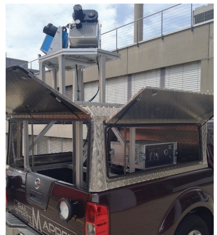
The RailMapper with two Z+F PROFILER® 9012
