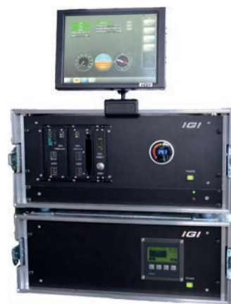
IGI Mobile Mapping control unit with uninterruptable power supply.
