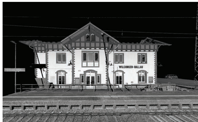
Point cloud of a railway station in Switzerland, scanned with a Z+F PROFILER® 9012 (Picture: IGI).
