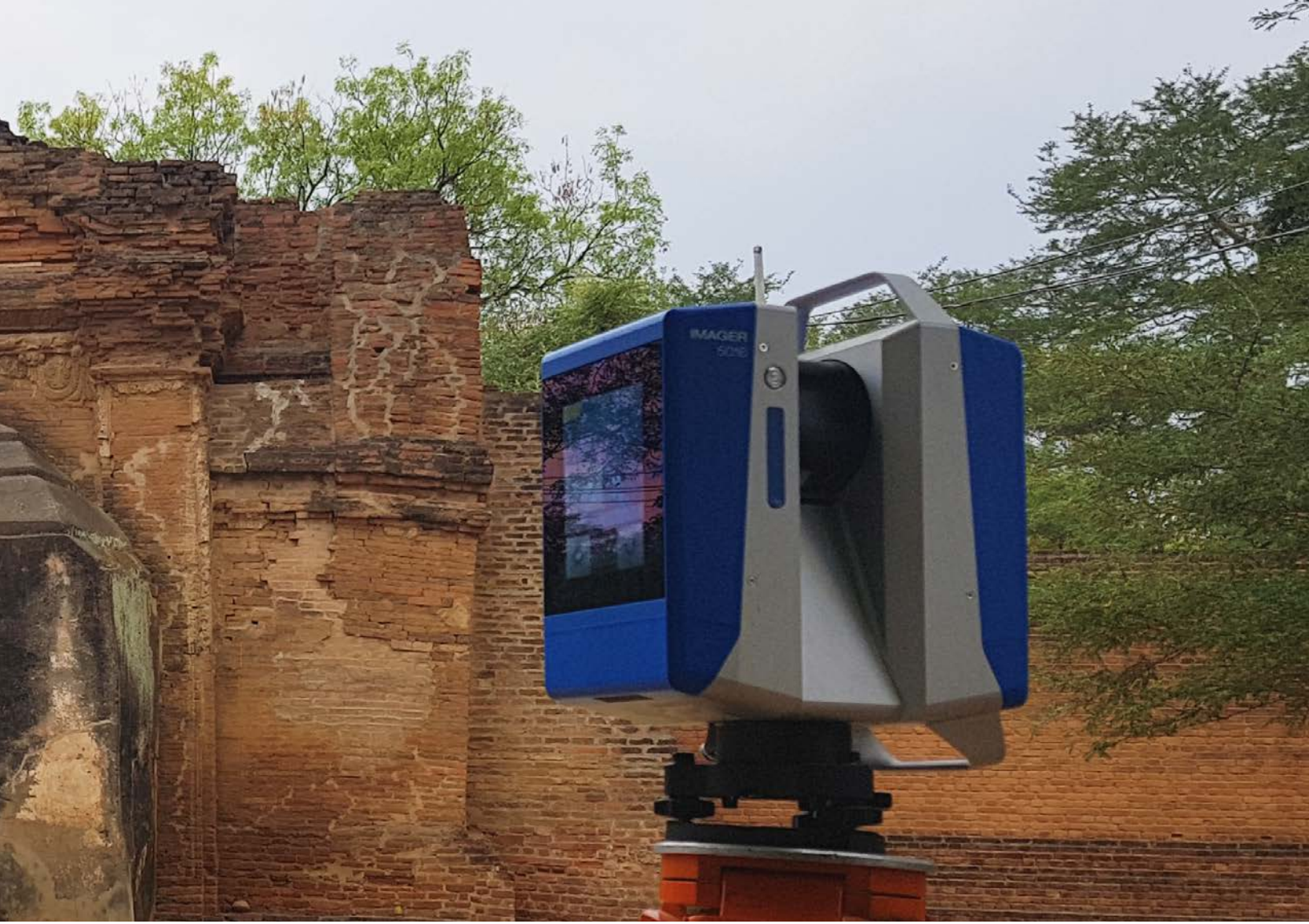
Multi-scanner-workflow with the Z+F IMAGER® 5016 during scanning the old city gate of Bagan
