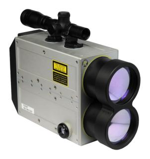
The *RIEGL* LD05-A80 is a multi-purpose laser distance meter based on precise time-of-flight laser range measurement. It uses state-of-the-art **digital signal processing** enabling precise distance measurement for complex multi-target situations even under bad visibility conditions. Digitizing the echo signal and subsequent analyzing allows multi-target distance measurements. Up to 5 target distances can be detected and provided for each laser shot.
